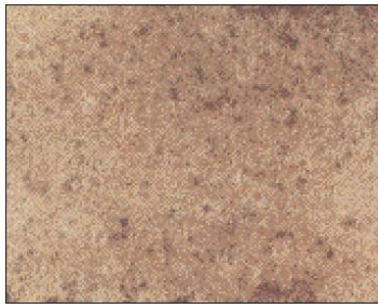
3CR12 PERFORMANCE AFTER 10 YEARS SERVICE IN MEDIUM TO SEVERE MARINE ENVIRONMENT
